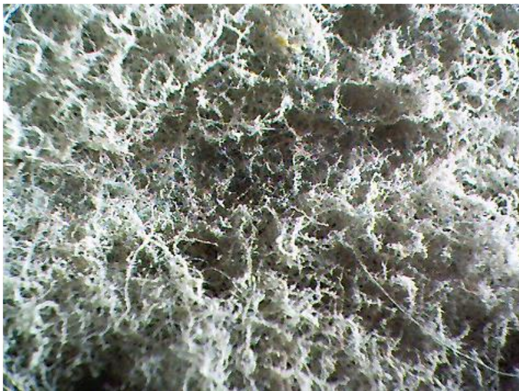
Photograph of particulate and fibrous materials collected after approximately six weeks of usage.
