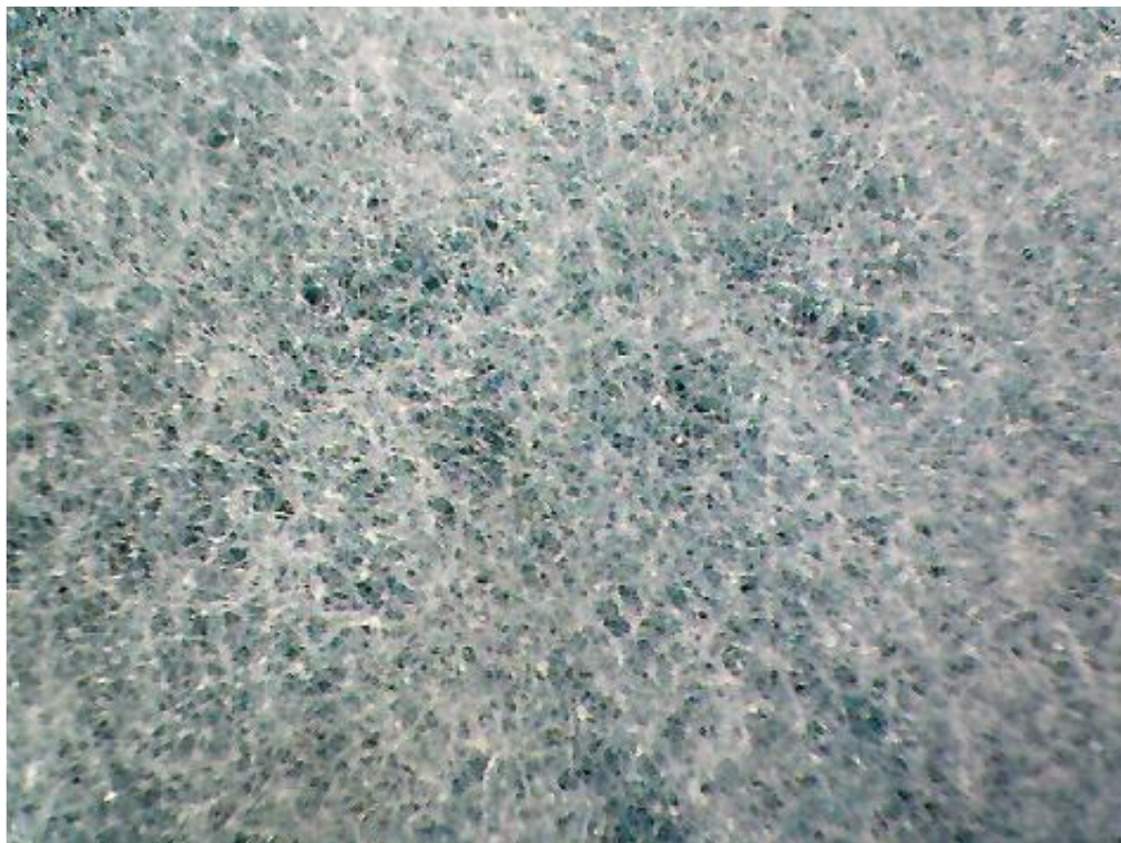
Photograph of original filter material, unused.
