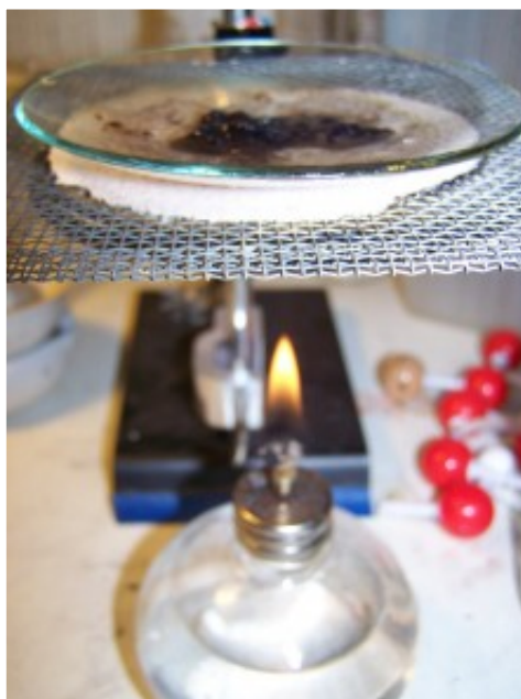
Drying the metallic residue from the electrolytic processing of the oral sample.
