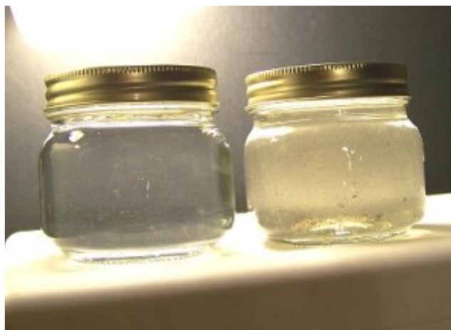
Concentrated Rain Sample under Study in this Report Distilled Water Reference on Left, Concentrated Rainfall to Right
