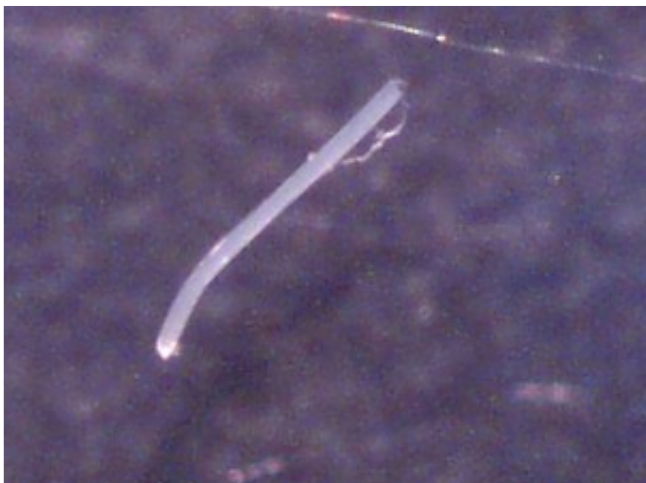
The same synthetic fiber shown above under the microscope at 60x, illuminated with black light (UV). Extreme fluorescence, but bears no similarities to earlier ground sample. Fiber diameter significantly greater than 1 micron, and by all appearances one of thousands of similar fibers (i.e., lint) in this residential environment.
