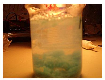
Approximately 24 hours into the electrolysis process. Significant precipitate formation at bottom of container. Fibers have been removed.
