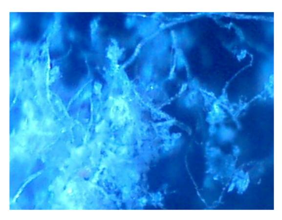
Magnification 200x Fibers and Crystal-Powder Form Collected from Ionizing Air Filter
