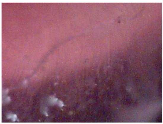
Interspersed transparent or colored larger fibers are occasionally visible. Colored fibers are usually blue or red. Blue fiber visible in this microphotograph. Wet slide. Magnification 200x.
